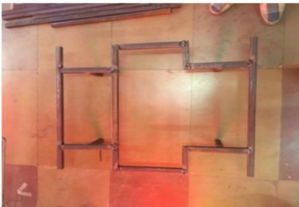
Figure4:-Completely welded chasis.
